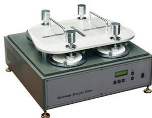
Figure 1: Martindale abrasion tester machine
